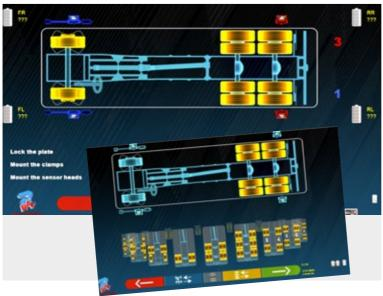
Vehicles with multiple axles can be measured simply and quickly. The guided procedure is easy to follow, even for less experienced operators.
