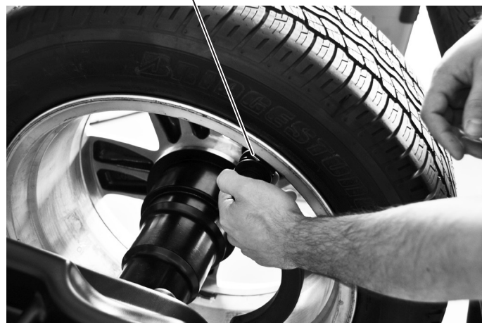
Fit weight on the position where pliers touches the wheel
