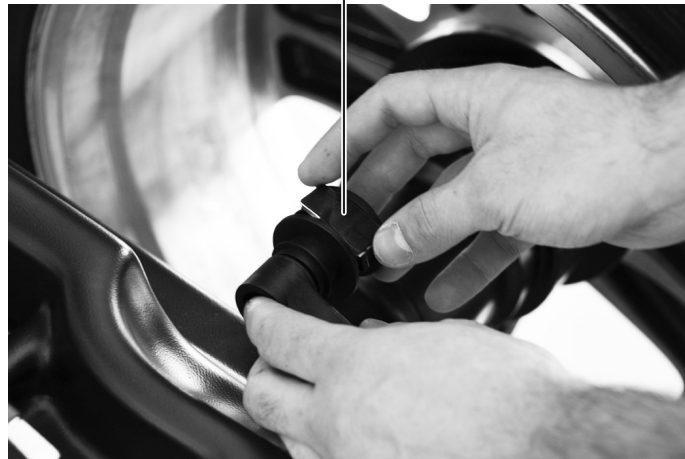
Fit the adhesive weight in the pliers of the gauge rod
