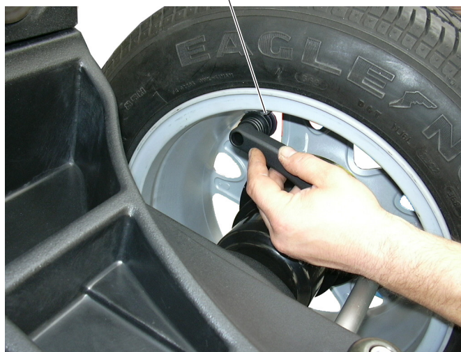
Fit weight on the position where pliers touches the wheel
