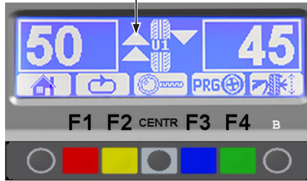
Arrows to help positioning in correction weight fitting point
