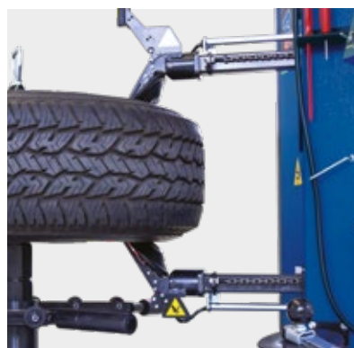
Double bead breaking discs system. The tyre bead is broken quickly and safely by two opposite synchronised discs.
