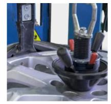
Upper mounting head of nonscratching material for damagefree work on the rims near the edge (zero stress effect).
