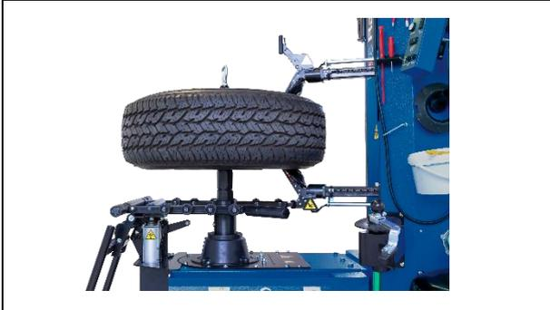
Tyre-changer-G1250.30\_Double bead breaking-DI-2
