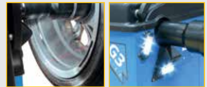
GAR 311 Laser pointer + double led light
